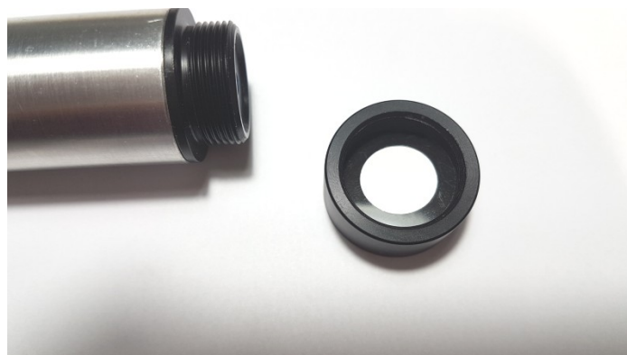
6 - The membrane can be easily unmounted unscrewing the top cap
