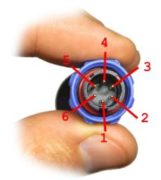
The waterproof 6 pins connector has got the following pinout:
